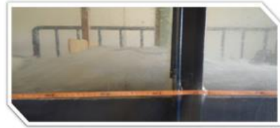
Fig.5. hydraulic jump controlled by a thin sill
