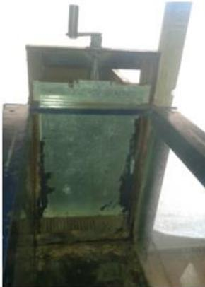
Fig. 2. Manual metal plate (bottom sluice gate).
