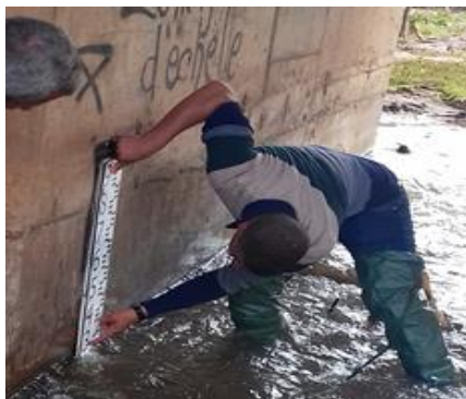
Photo sheets 1: installation and monitoring of the limnimétrique scale
